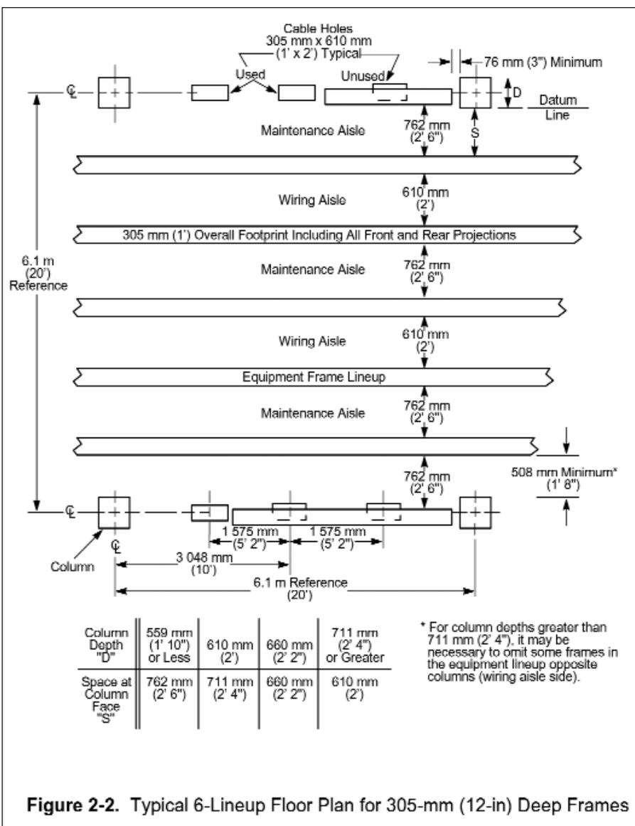
Figure 2-2. Typical 6-Lineup Floor Plan for 305-mm (12-in) Deep Frames
